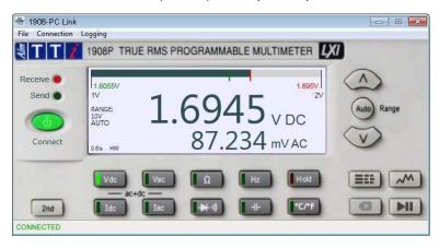
The application provides remote access to the instrument using a pointand-click interface arranged similarly to the actual instrument.
